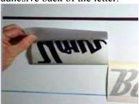
12. While holding the lettering out to avoid contact with the transom, apply firm pressure with the edge of your squeegee (hard plastic applicator enclosed with your order) starting at top and working outward toward each edge. Be careful to let the adhesive letters touch only as the squeegee presses it against the surface. Continue in the same manner across each section of the hinged vinyl letters.
