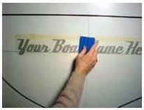
14. Starting at the corner slowly peel each section of the tape that covers the vinyl letters back and flush against the surface of the transom. Do not pull straight out from the transom. Letters may pull off.
