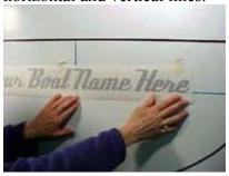
10. When you are satisfied with the positioning, apply a horizontal tape "hinge" along the top edge of the vinyl boat letters over the tape tabs.
